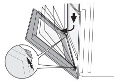
Hold the door strip (B) on both sides, align it with the inner edge of the door and press the door strip (B) into the upper edge of the door.
